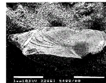
Fig. 5. Irregular piece broken from a crystal of SrTiO 3 used to measure the spectra in Fig. 6.
